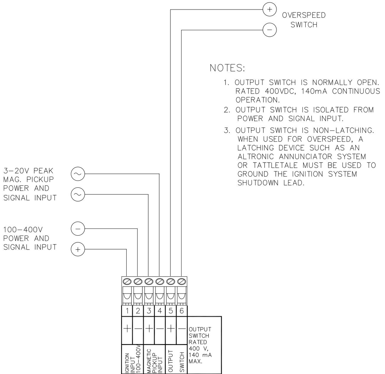
FIG. 4 DTHO-1201/3201 WIRING DIAGRAM
