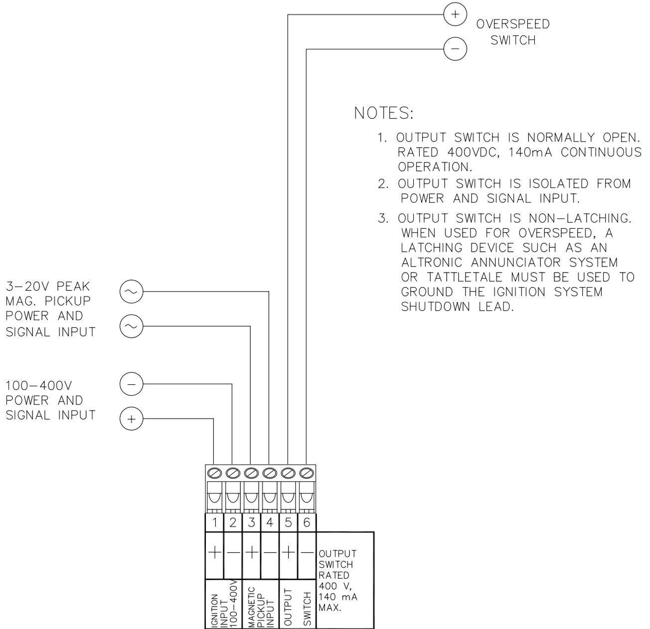
FIG. 4 DTHO-1201/3201 WIRING DIAGRAM
