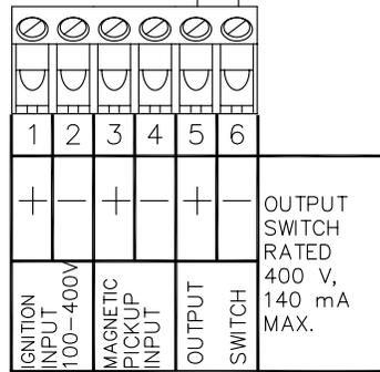
FIG. 9 DTHO-1201/3201 WIRING DIAGRAM - TATTLETALE
