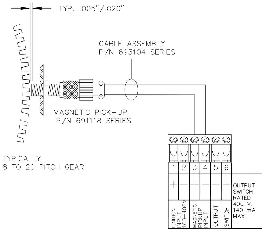
FIG. 7A DTHO-1201/3201 WIRING DIAGRAM INTRINSICALLY SAFE FOR NEGATIVE GROUND IGNITIONS
