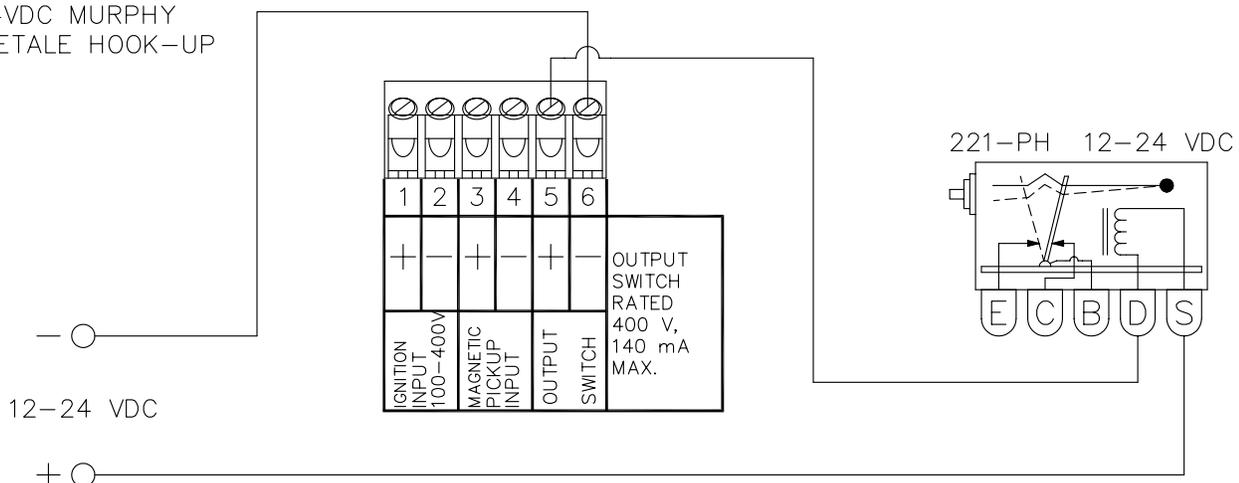
FIG. 10 DTHO-1201/3201 WIRING DIAGRAM - PNEUMATIC VALVE
