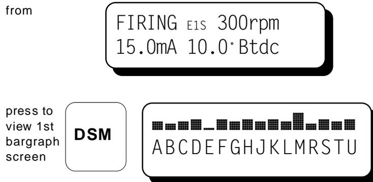
The second bargraph screen shows the difference between the spark reference number for each ignition output and the engine or group average. Scaling for this graph is determined by high and low from engine alarm values. The engine or group average is shown as a single narrow line across the middle of the character field. Bars extend up or down from narrow line to indicate relative deviation plus or minus of each cylinder from the engine or group average.
