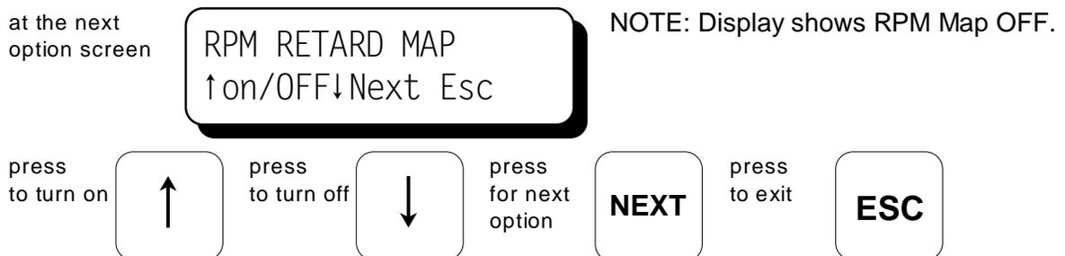
6.4 The Next mode selection can enable or disable the additional retard value controlled by the serial port. To use this option reference form CPU-2000 PI.
