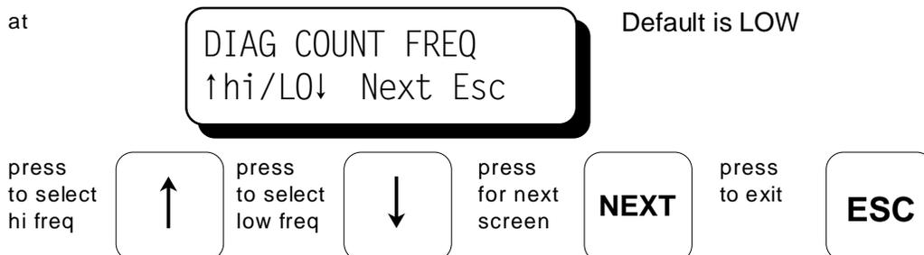
9.13 WITH OPTIONAL DIAGNOSTIC MODULE ONLY: The next screen is used to select the RPM at which to permit the update of the MIN/MAX historical cylinder data array. This feature is provided to avoid the update of the MIN/MAX values when the engine is running below normal loaded conditions.
