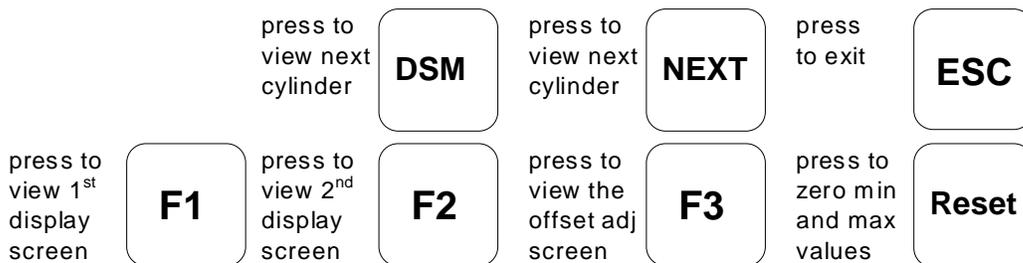
12.6 The offset adjustment screen (F3) permits the operator to use an offset adjustment to the spark reference number (+/- 15 counts) to compensate for minor variations in reference numbers between individual coils of the same type and voltage demand. To initialize all offset values to zero from this screen, press "Reset".
