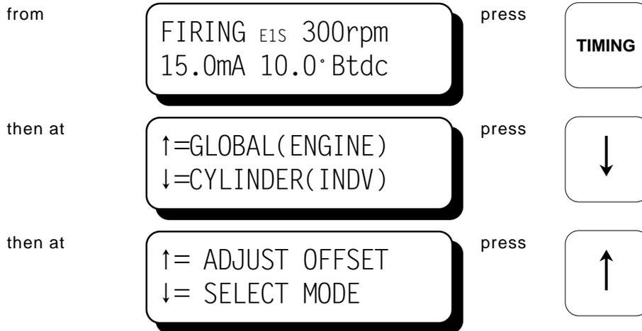
7.3 The individual timing adjustment screen identifies the primary output(s) to be adjusted, and the degrees of offset in use for the output(s). In some cases, two outputs are controlled together.
