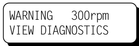
10.3 If the Alarm Out switch is being used to turn on an audible alarm or flasher, the user can acknowledge the alarm to silence the alarm. After viewing faults or warnings, the user would then reset and re-arm the ignition system after the faults or warnings have been addressed.
