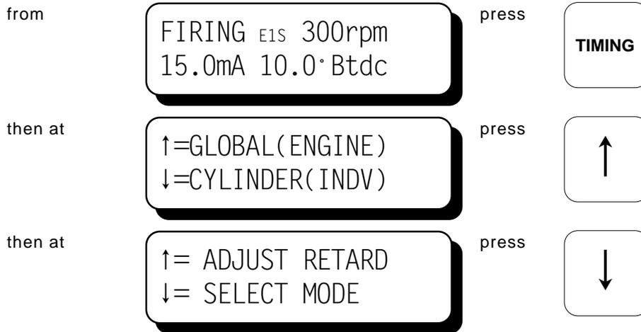
6.2 The first mode selection can enable or disable the pre-configured retard curve controlled by the 4-20 mA current loop input. The choices are ON and OFF, with the active selection displayed in capital letters. To configure the 4-20 mA curve, reference form CPU-2000 PI. When the current loop is on, the home screen displays the current loop value (xx.x mA). When the current loop is off, the display reads (xx.x ma).
