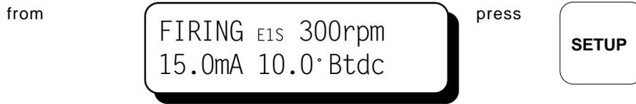
9.2 The first setup screen permits the operator to enable or disable the Multi-Strike feature.
