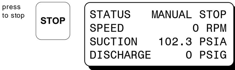
NOTE: The stop function can also be implemented remotely by using the external STOP input available on the Terminal Module. The behavior of the Controller and display will be identical to that obtained by pressing the local STOP key on the Display Module.
