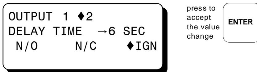
The selection arrow replaces the diamond indicating a change can be made. The selected output switch can be configured for N/O (normally open), N/C (normally closed), or IGN (ignition module 691124).
