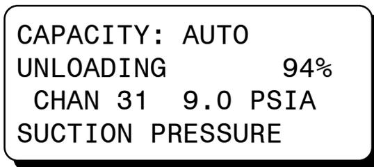
Indicates that the current value of channel 31 is below the desired setpoint by more than the allowable deadband and that the output of the controller is being changed to decrease the load which will eventually cause the suction pressure to increase towards the setpoint.
