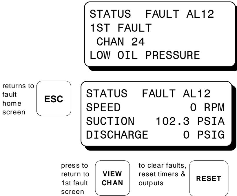
NOTE: The reset function can also be implemented by using the external hardware. RESET / AUTO START input available on the Terminal Module. The behavior of the Controller and display will be determined by the programming selections made when configuring the unit.
