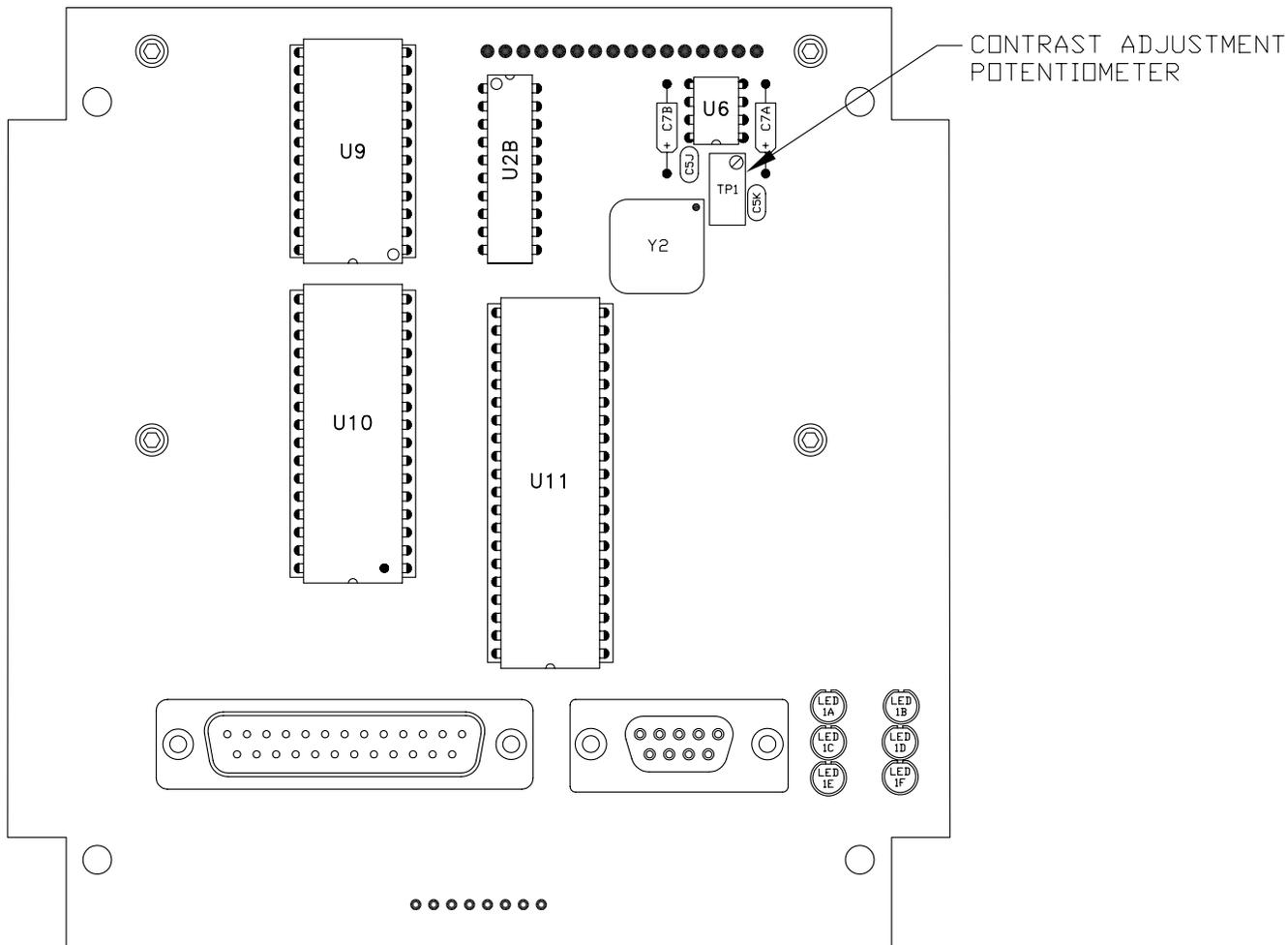
1. TO ADJUST LCD DISPLAY CONTRAST RATIO: USE AN ADJUSTING TOOL AND TURN THE POTENTIOMETER CLOCKWISE TO LIGHTEN THE CONTRAST RATIO OR COUNTERCLOCKWISE TO DARKEN THE CONTRAST RATIO. TO SET THE POTENTIOMETER BACK TO THE FACTORY SETTING; WITH THE DISPLAY MODULE AT AN AMBIENT TEMPERATURE OF APPROXIMATELY 65°F TO 77°F (18°C TO 25°C), TURN THE POTENTIOMETER COUNTERCLOCKWISE THREE TO THREE AND ONE HALF TURNS. THE DISPLAY SHOULD THEN BE AT A DESIRABLE CONTRAST RATIO.
