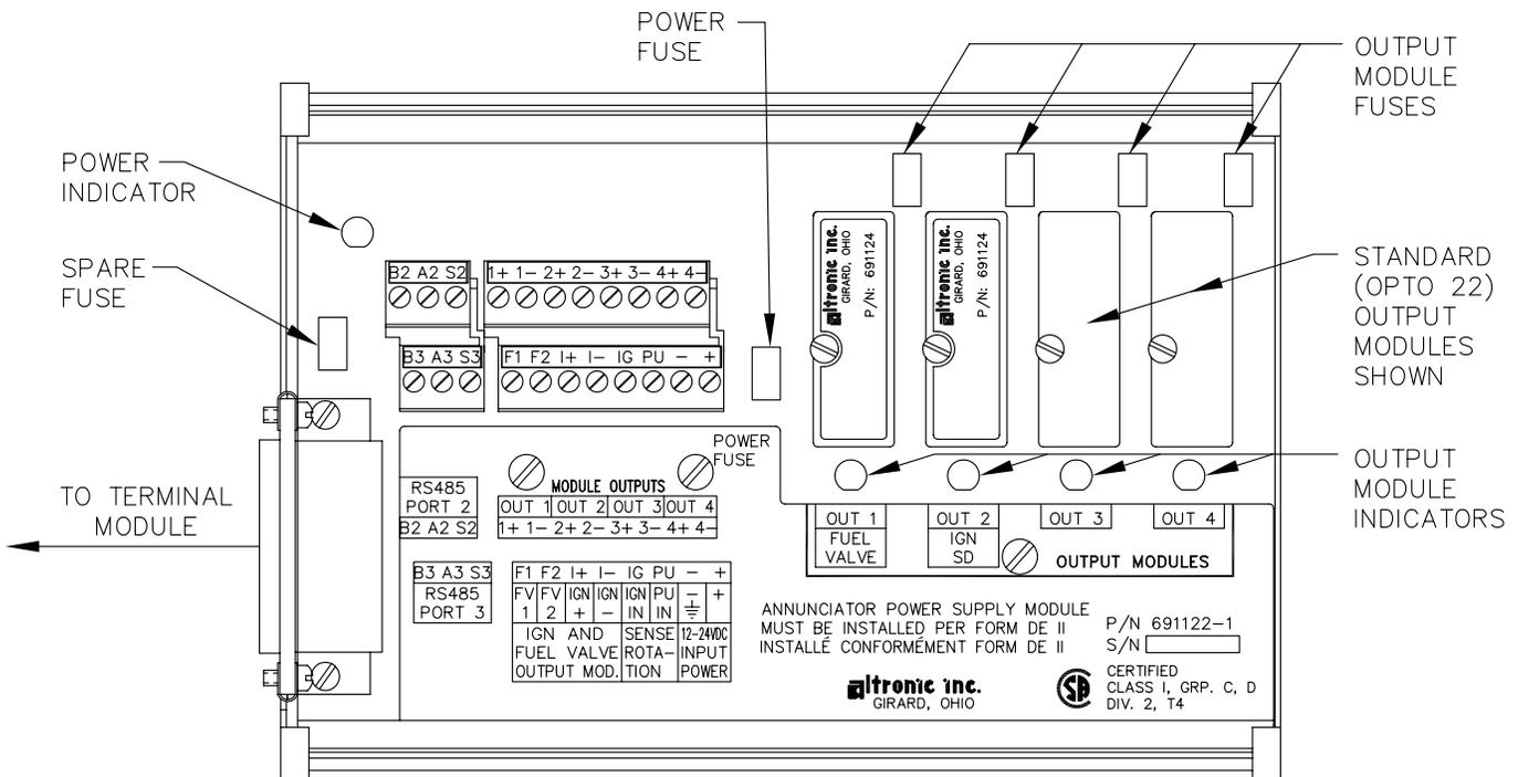
**FUSES:** FUSES ARE REPLACEABLE 6.3 AMP, P/N 601653.
