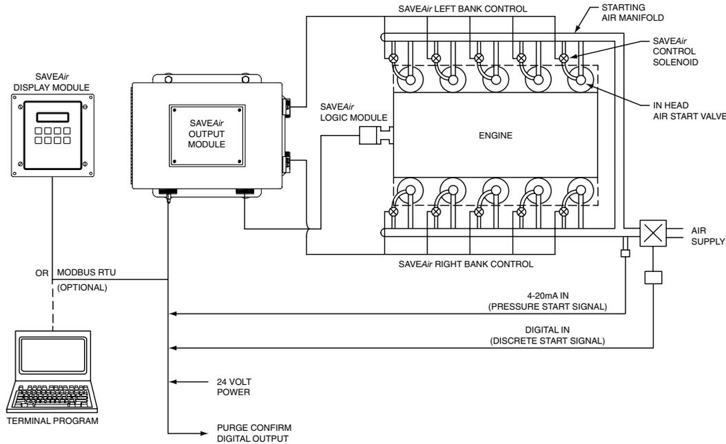
The SaveAir Electronic Air Start System is designed to be retrofit to almost any engine utilizing the air-in-head starting method. A description of the function of the major components and their integrated operation appears below:
