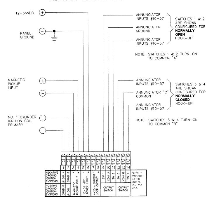
NOTE: FOR INTRINSICALLY SAFE OPERATION, POWER THROUGH A CSA CERTIFIED ZENER BARRIER RATED 30 VOLTS MAX., 1200 MIN. THE NO. 1 CYLINDER IGNITION COIL PRIMARY INPUT MUST BE CONNECTED THROUGH AN ALTRONIC BARRIER 690 107 OR 690 108. FOLLOW THE INSTALLATION INSTRUCTIONS SUPPLIED WITH THE BARRIERS. THE MAGNETIC PICKUP INPUT MUST BE FROM AN ALTRONIC 691 118 PICKUP.
