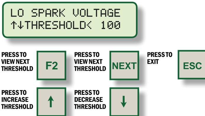
**12.3** If the **CAVG** reference number of a cylinder is above the **HIGH SPARK VOLTAGE** threshold, a diagnostic warning for that cylinder will occur. When a high spark warning is present, the ignition energy will automatically be increased to at least **E2**. This test will identify a high voltage demand condition which may result, for example, from worn spark plugs or poor air-fuel ratio control. To disable, set to **255**.
