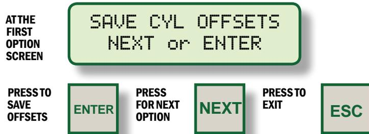
**8.3** The **NEXT** mode function can be used to reset all cylinder offset values back to zero (both temporary memory and EEPROM memory).
