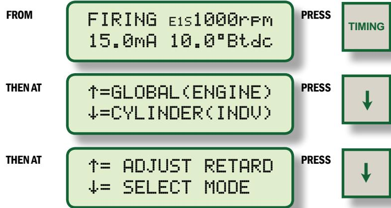
**8.2** The first function is used to save the current (temporary) individual offsets to EEPROM memory. When this is done, the ignition will load these offset settings every time the engine starts or reset is pressed. **REFERENCE SECTION 7.0** to adjust individual (temporary) offsets.
