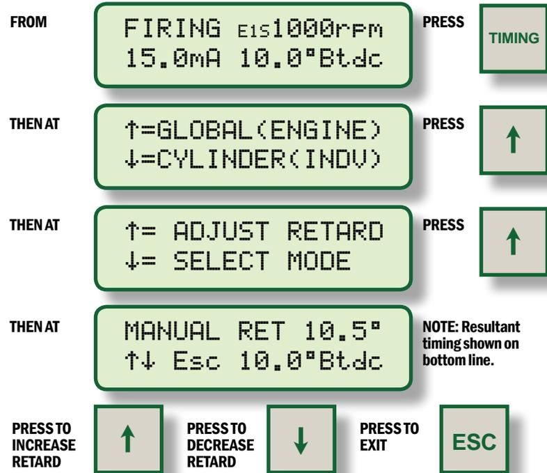
**5.3** The increment of timing change is dependent on the number of holes or teeth being sensed. The minimum timing change is defined as follows.
