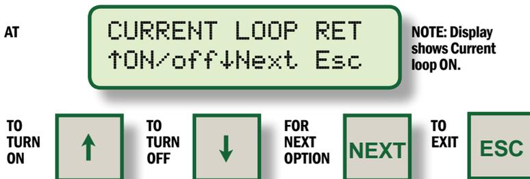
6.3 The Next mode selection can enable or disable the pre-configured retard curve controlled internally by engine RPM. To configure the RPM retard curve, reference form CPU-95 PI.
