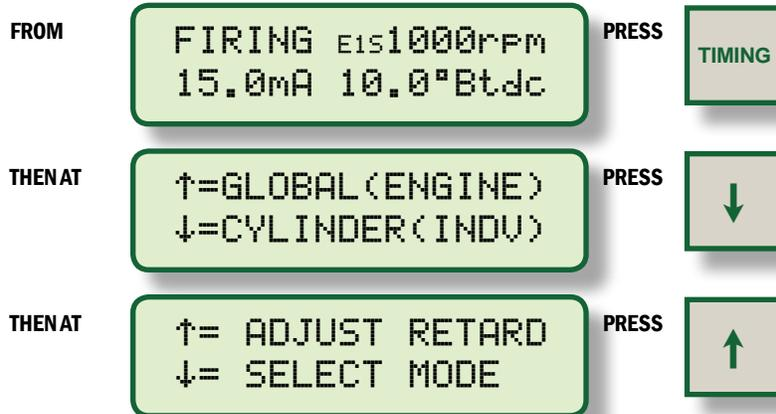
**7.3** The individual timing adjustment screen identifies the primary output to be adjusted, and the degrees of offset in use for the output.
