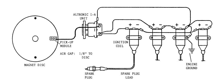
NOTE: SEE THE WIRING DIAGRAMS AND DISC AND PICK-UP MODULE INSTALLATION DRAWINGS FOR THE SPECIFIC APPLICATION.
