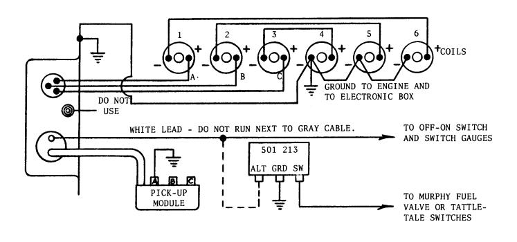
ALTRONIC I-6 WIRING DIAGRAM - 6 CYLINDER, 4-CYCLE FIRING ORDER 1-4-2-6-3-5
