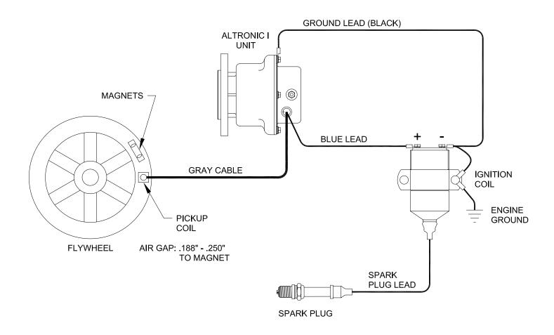
NOTE: SEE THE TIMING SETTING CHART (PG. 2) AND WIRING DIAGRAMS ON THE FOLLOWING PAGES FOR THE SPECIFIC APPLICATION.
