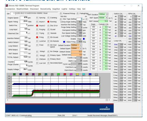
PLEASE NOTE: The terminal program has been revised to NGI-1000RC for communication to NGI-1000RC Ignition modules after SN 2001. The screen shot provided here reflects the significant changes. Note that Node ID has been changed from 1 to 11 to differentiate between FW versions. Also, Green background parameters are RAM based and can be freely written. Orange background parameters are used to specify preload values which are copied to the green RAM-based values at power up and upon re-start.
