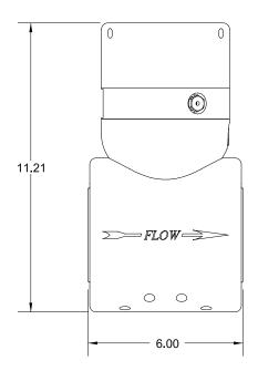
AGV5 GAS METERING VALVE ENVELOPE DRAWING, 2" CLASS 150 FLANGE
