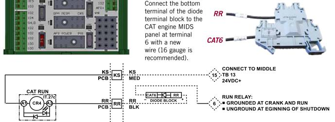
2. All new Flex Panels with RevO or Rev1 PCBs will be shipped with an external diode terminal block. The diode block can be placed into service by either the packager or the end-user when interfacing with a CAT 3300B engine MIDS panel by following the above directions.
