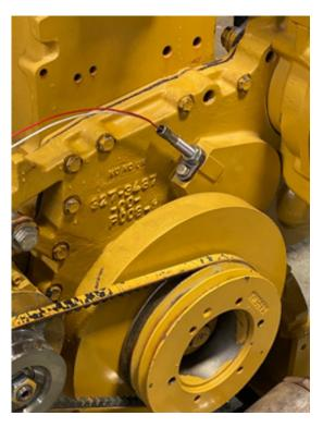
Engine Front cover re-assembled
