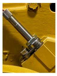
Pickup Bracket with PU mounted (shim washer for mounting bolt is provided). ½ turn of the pickup from touching the disc will yield the proper 0.020" gap.
