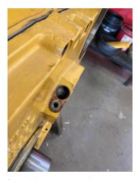
Cam Pickup Mounting Hole
