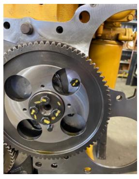
The trigger gear is shown removed. The three holes and one dowell are used to mount the disc. The dowell indexes the disc so that it cannot be incorrectly mounted. Original bolts re re-used.
