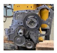
Cover removed showing original cam trigger gear
